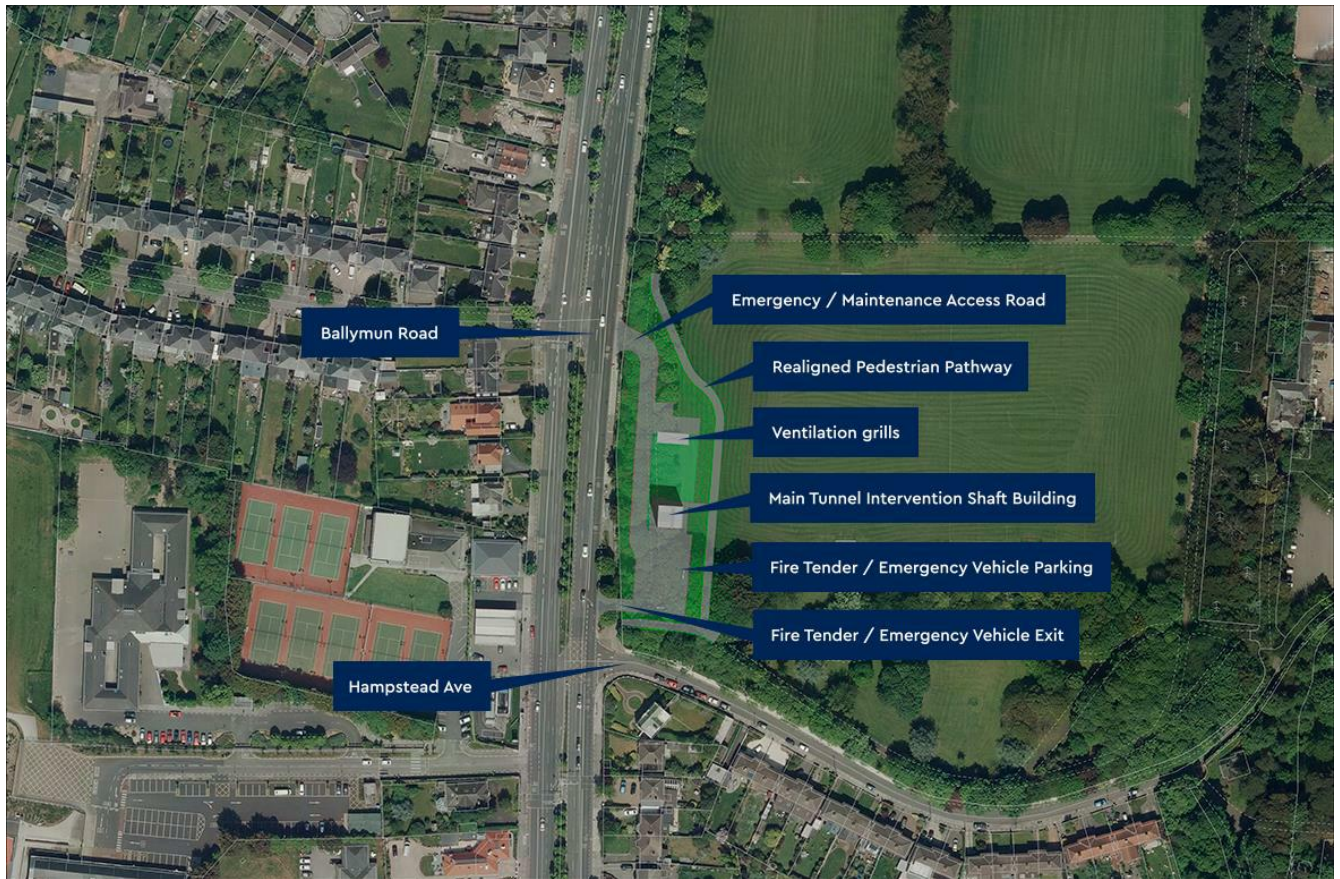
Figure 4.10: Road Access and Emergency/Maintenance Vehicle Parking
